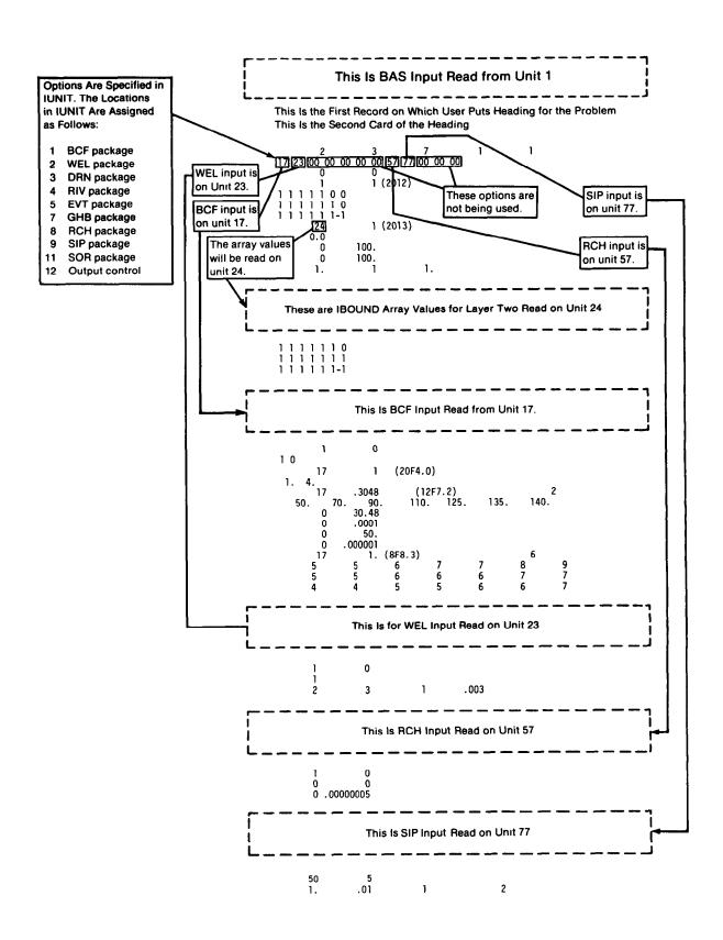
Figure 18.—Sample input data showing role of the IUNIT array.
