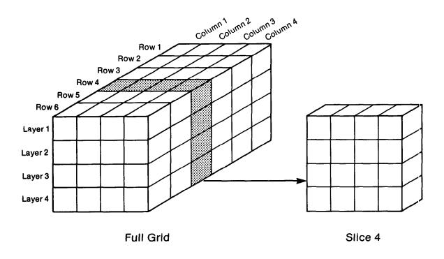
Figure 54.—Division of the three-dimensional model array into vertical slices for processing in the SSOR package.
