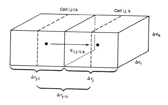
Figure 4.—Flow into cell i,j,k from cell i,j-l,k.
