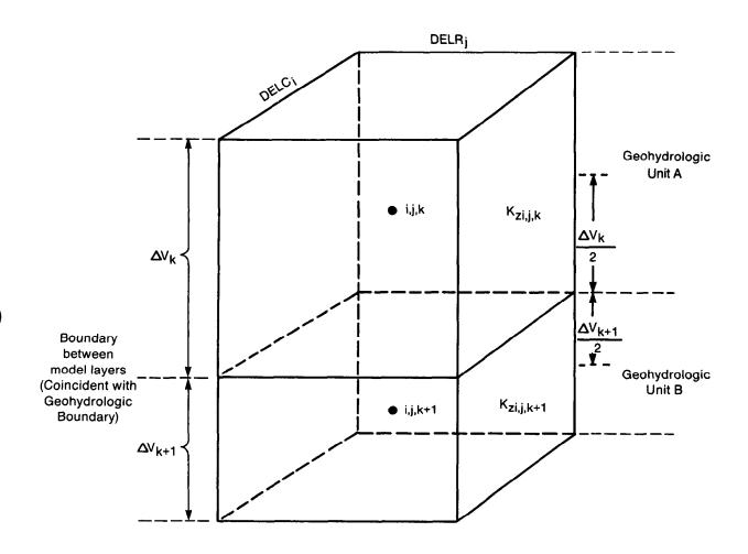
Figure 27.—Diagram for calculation of vertical leakance, Vcont, between two nodes located at the midpoints of vertically adjacent geohydrologic units.
