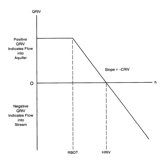
Figure 36.—Plot of flow, QRIV, from a stream into a cell as a function of head, h, in the cell where RBOT is the elevation of the bottom of the streambed and HRIV is the head in the stream.
