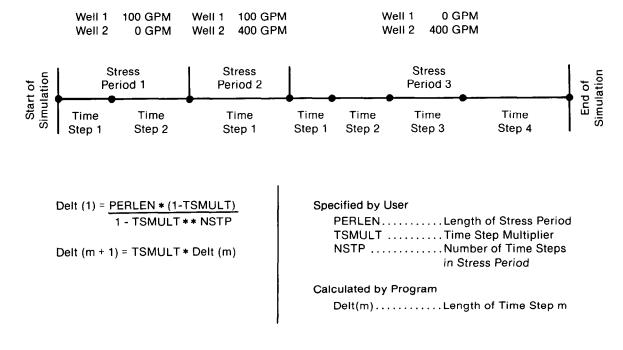
Figure 21.—Division of simulation time into stress periods and time steps.
