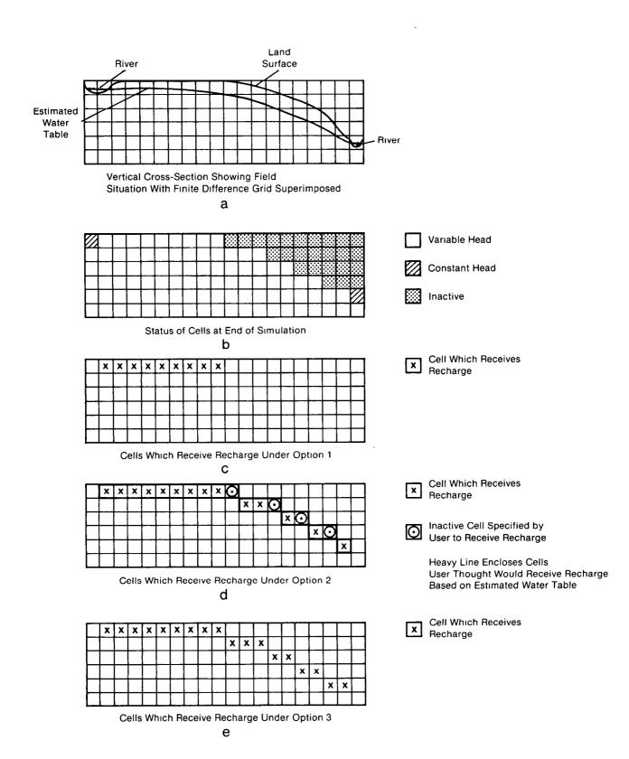
Figure 38.—Hypothetical problem showing which cells receive recharge under the three options available in the Recharge Package.
