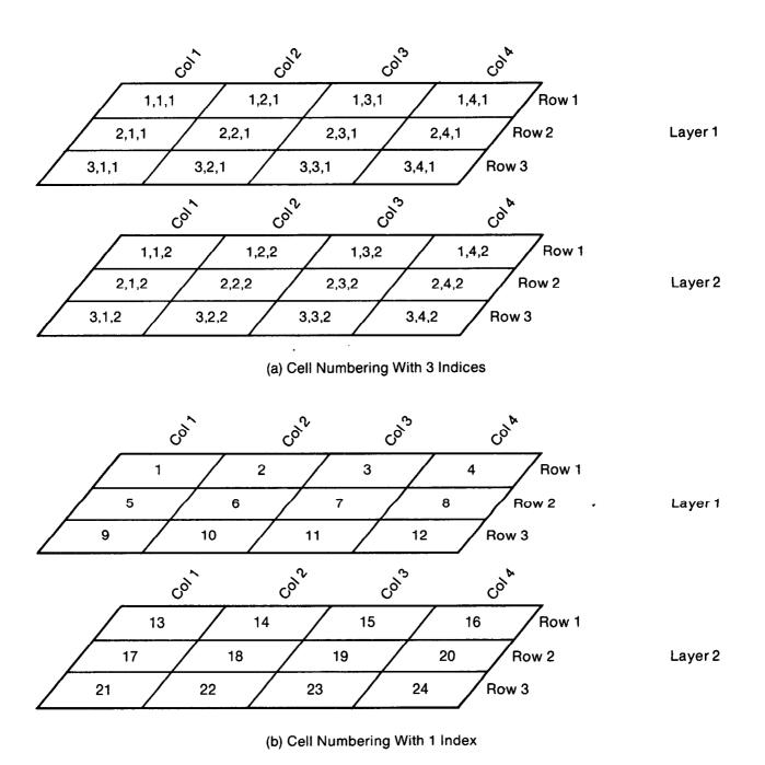
Figure 53.—Cell numbering schemes for a grid using three indices and using one index.
