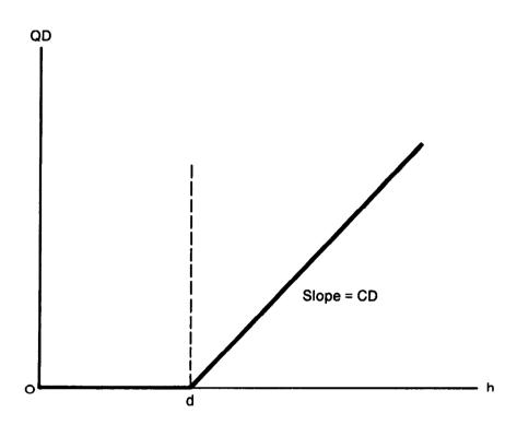
Figure 41.—Plot of flow, QD, into a drain as a function of head, h, in a cell where the elevation of the drain is d and the conductance is CD.
