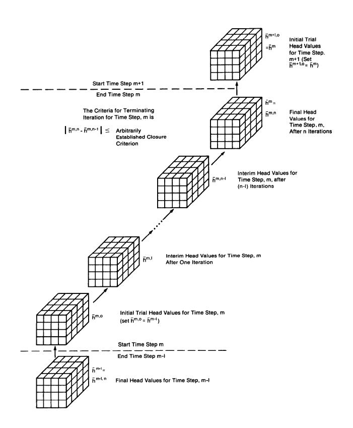
Figure 7.—Iterative calculation of a head distribution.
