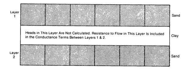
Figure 12.—A cross section in which a low conductivity unit is represented by the conductance between model layers.
