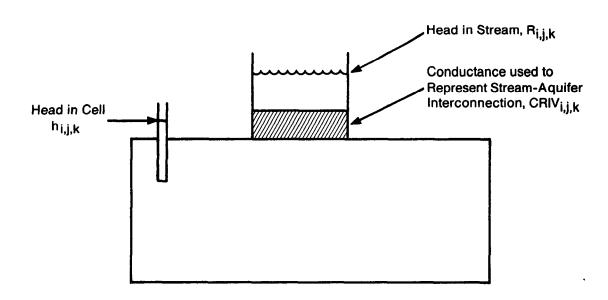
Figure 5.—Conceptual representation of leakage through a riverbed into a cell.
