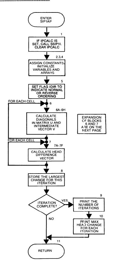
Single Cell Index: In this module, a single index is used to identify each cell. This is in opposition to the three indices (I,J,K) used in most other modules.
