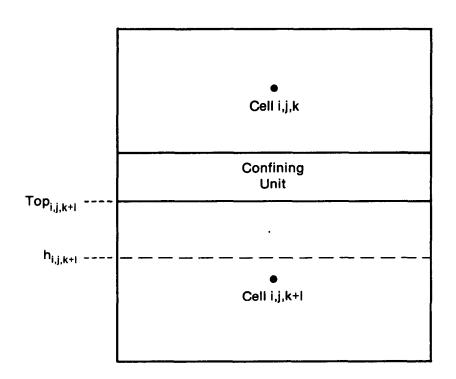
Figure 29.—Situation in which a correction is required to limit the downward flow into cell i,j,k+1, as a result of partial desaturation of the cell.
