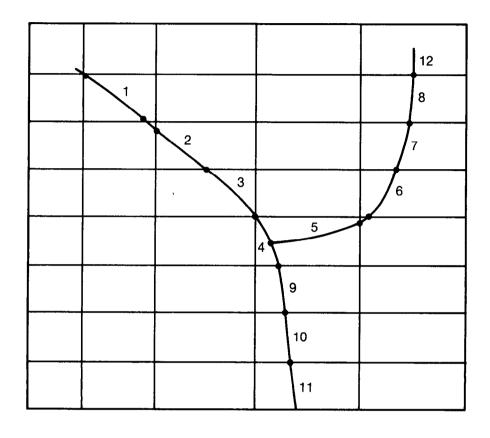
Figure 32.—Discretization of a stream into reaches. Some small reaches are ignored.
