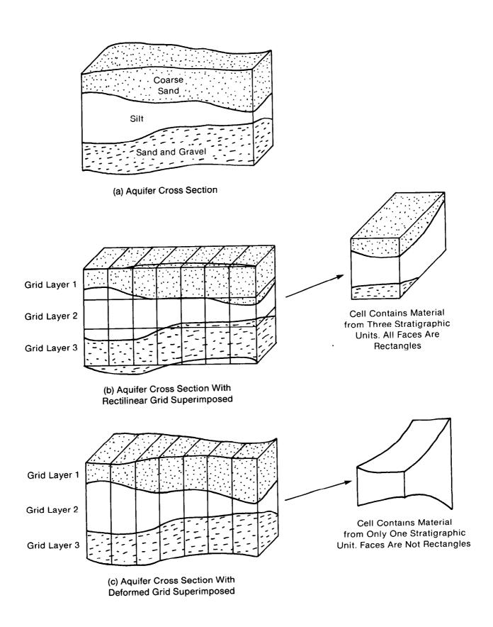
Figure 9.—Schemes of vertical discretization.
