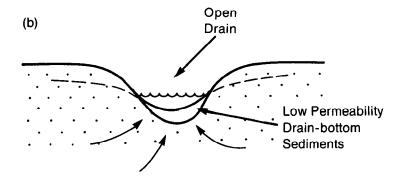
Figure 40.—Factors affecting head loss immediately around a drain: (a) buried drain pipe in backfilled ditch and (b) open drain.
