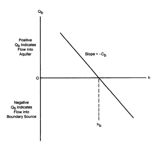
Figure 45.—Plot of flow, Q<sub>b</sub>, from a general-head boundary source into a cell as a function of head, h, in the cell where h<sub>b</sub> is the source head.
