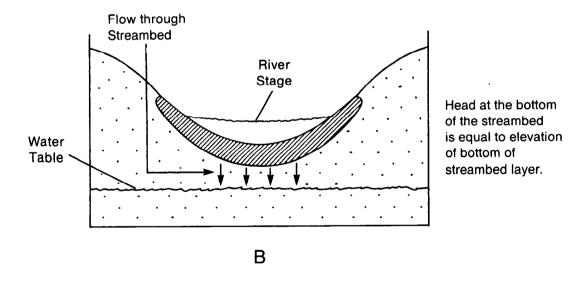
Figure 35.—Cross sections showing the relation between head at the bottom of the streambed layer and head in the cell. Head in the cell is equal to the water-table elevation.
