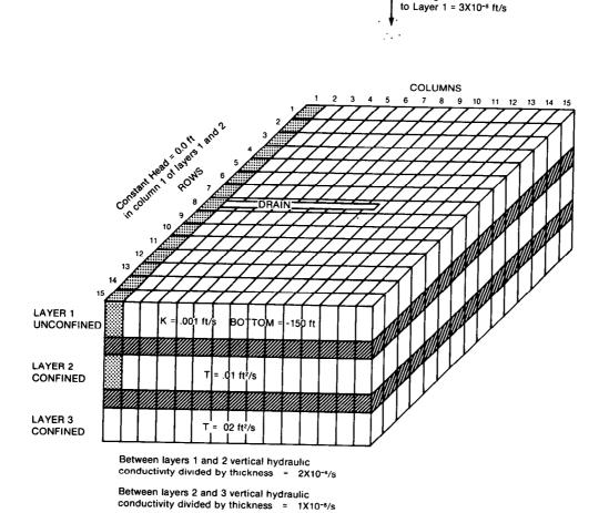
Setting starting heads equal to 0.0, the program was run to get a steady-state solution. The Strongly Implicit Procedure was used to solve the system of difference equations: the error criterion was set at 0.001 feet, the acceleration parameter was set to 1.0, and the maximum number of iterations was set equal to 50. A seed of 0.001 was specified for use in calculating the iteration parameters; 31 iterations were needed to close.
