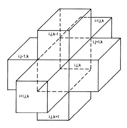
Figure 3.—Cell i,j,k and indices for the six adjacent cells.
