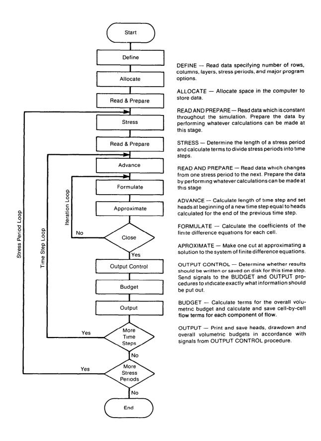
Figure 13.—Overall program structure.
