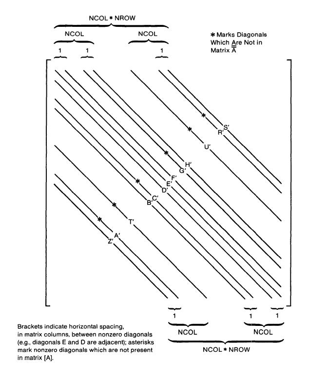
Figure 50.—Structure of matrix [A+B] showing nonzero diagonals.
