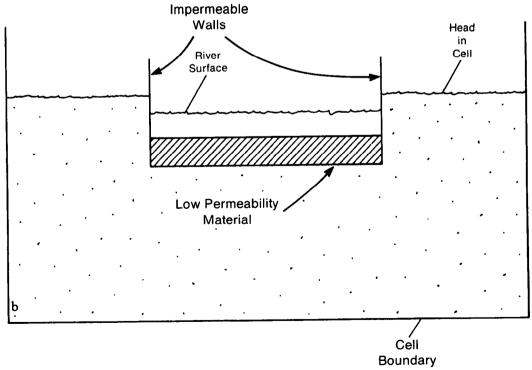
Figure 33.—(a) Cross section of an aquifer containing a stream and (b) Conceptual representation of stream-aquifer interconnection in simulation.
