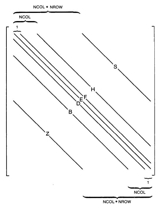
Brackets indicate horizontal spacing, in matrix columns, between nonzero diagonals (e.g., diagonals E and F are adjacent).
