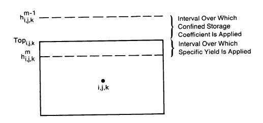
Figure 30.—A model cell which uses two storage factors during one iteration.
