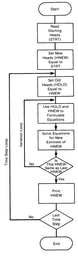
Figure 20.—Flow of head distributions during a simulation.
