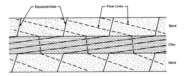
Figure 10.—Possible pattern of flow in a cross section consisting of two high conductivity units separated by a low conductivity unit.
