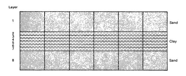
Figure 11.—A cross section in which a low conductivity unit is represented by six model layers.
