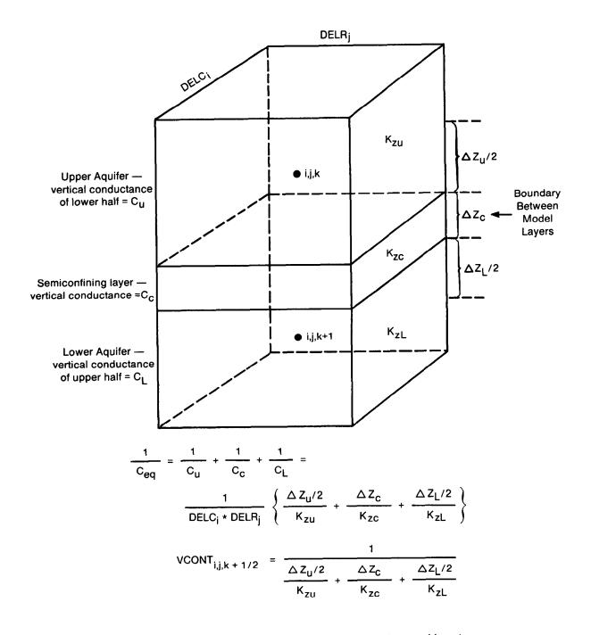
Figure 28.—Diagram for calculation of vertical leakance, Vcont, between two nodes located at the midpoints of aquifers which are separated by a semiconfining unit.
